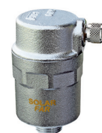
Fig.1 If there is no air in the circuit, water inside the air vent valve keeps the float in such a position as to close the shutter.
